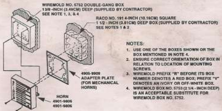
Figure 10. Surface Mounting of Mechanical Horns
