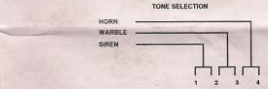
Figure 12. Selecting a Tone for Electronic Horn Model 4901-9809 or 4901-9810
